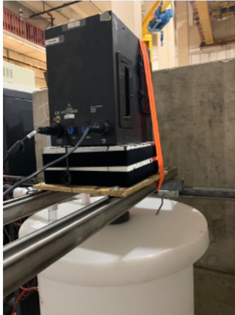
Figure 4.2: An angled view of the 85 mm \times 30 mm HPGe detector (crystal volume not visible) shielded by four white painted lead bricks (8" \times 4" \times 2") sitting atop of a half inch thick square of plywood. The detector sits 20 cm above the 114 L inventory tank. 2-inch-wide black Velcro straps ensure stability of the bricks while an orange ratchet strap secures the detector to the unistrut structure
