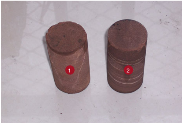
Fig. 3 Fractured sandstone specimens after uniaxial compression
