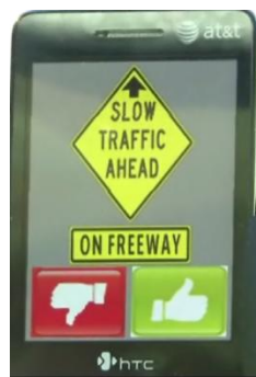
Figure 3.1. The NT Client warning display screen; the sentence “Slow traffic ahead” is voiced once while the above screen is displayed for 45 seconds.
