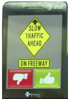
Figure 4.4. The user interface of the NT Smartphone application allowed us to capture, in real-time, the driver's feedback to the alert by tapping on the thumbs-up or thumbs-down buttons
