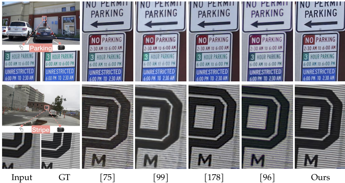
Figure 3.4: Our 4x zoom results show better perceptual performance in super-resolving distant objects against baseline methods that are trained under a synthetic setting and applied to processed RGB images. From left to right are: input, ground truth, Johnson et al. [75], SRResnet [99], ESRGAN [178], LapSRN [96] and ours.
