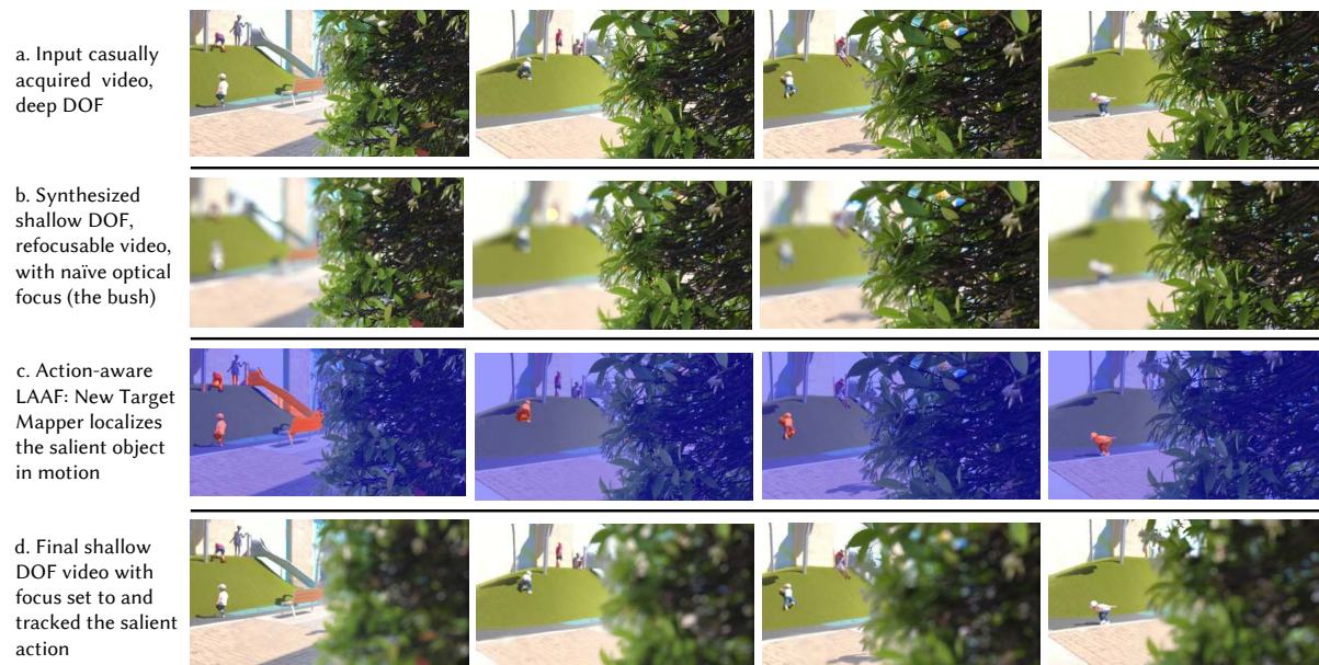
(4E) Action-aware video auto-focus. (Row 1) Input video shows children playing in the background and plant in foreground, optically focused on foreground. (Row 2) Naïve synthetic SDOF video would blur out the action in the background, because the input video is optically focused on the foreground. (Row 3) Intersection of visual saliency mapping and motion detection mapping isolates action of children in the background. (Row 4) The resulting video is autofocused on the background.
