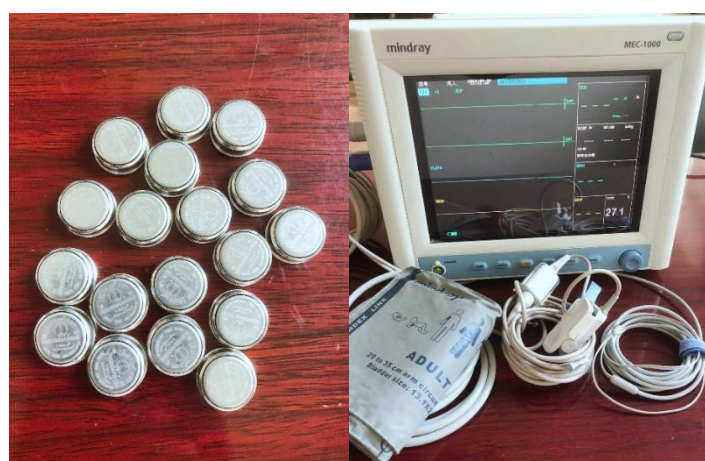
Figure 4 Diagrams of wireless temperature sensors and the physiological monitor
