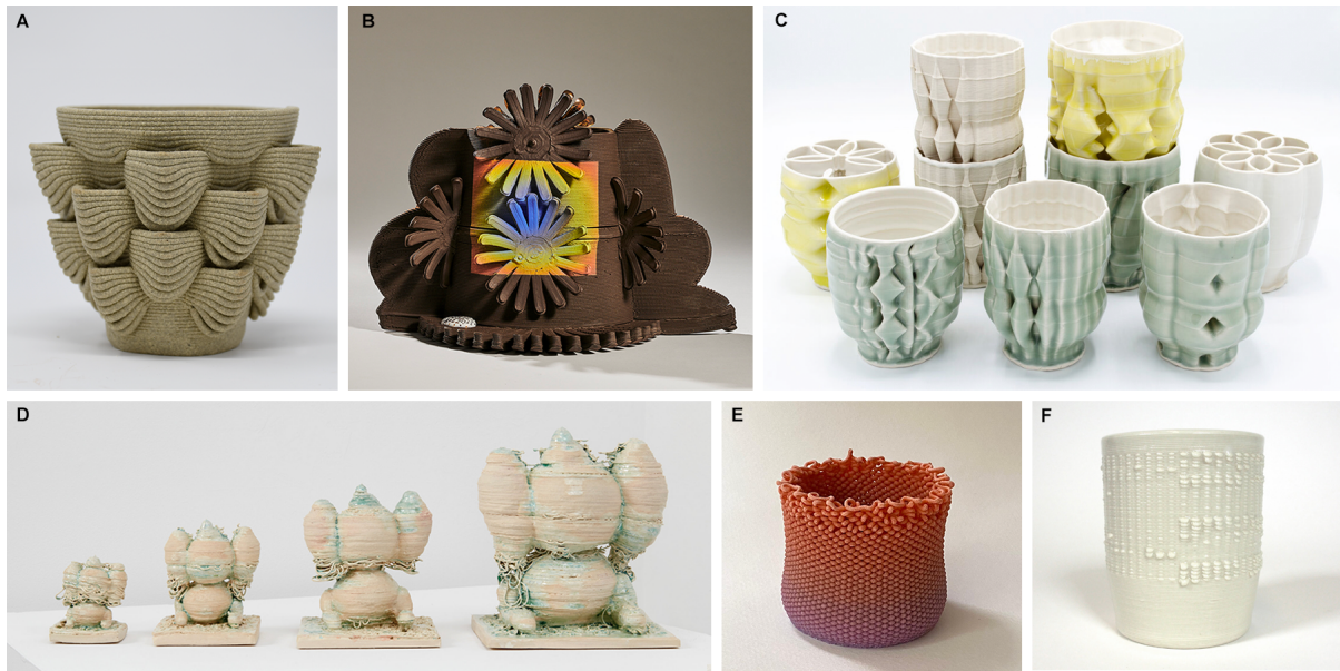
Figure 2.1: Notable work in the clay 3D printing field that exemplifies common textural and design elements. A) Researcher Sam Bourgault creates mathematically defined cups where the toolpath extends past the vertical edge of the form to create unsupported drooping loops [12]. B) Artist Jolie Ngo prints multiple vertically extruded forms and hand assembles them into complete works [38]. C) Artist Bryan Czibesz creates geometrically evolving surface textures via unique toolpathing [39]. D) Artist Eun-Ha Paek hand builds forms that she scans and re-prints [40]. E) Researcher Leah Beuchley creates irregular surface patterns by excessively increasing the z height between layers [41]. F) Researcher, Audrey Desjardins, and artist, Timea Tihanyi, teamed up to encode audio data in the toolpath of ceramic cups. [13].
