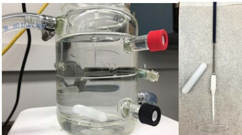
Fig. 40. Stirred beaker, left, stirrers, right.
