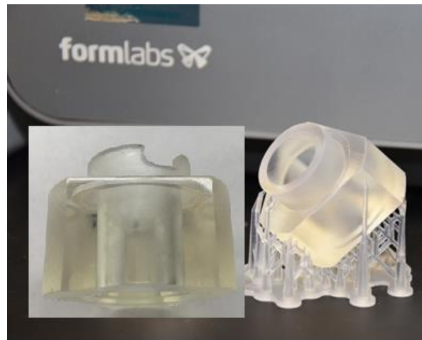
Fig. 17. 3D printed Robatel BXP012 housing.
