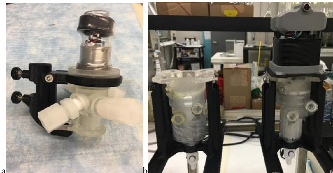
Fig. 20. ANL contactors. a) 10 mm. b) 20 mm (extended mixing zone to the left).
