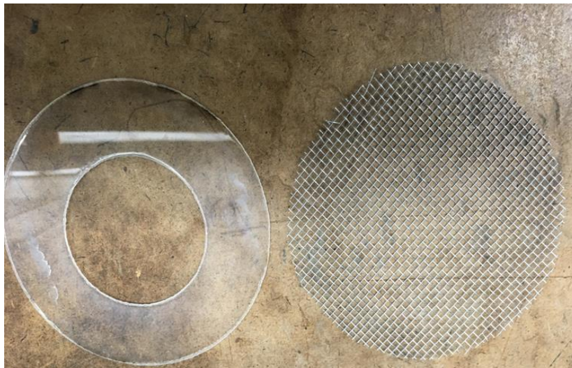
Fig. 49. Aluminum mesh, right, used in the high RPM experiment and a thin layer of PMMA, left, used in the interfacial area reduction experiment
