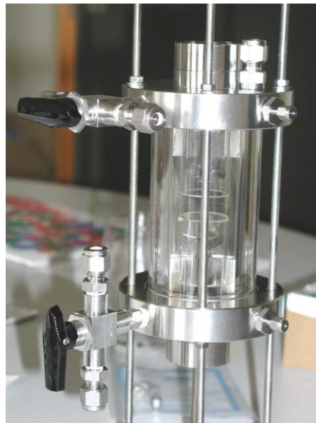
Fig. 41. The Nitsch cell designed at the Karlsruhe Institute of Technology
