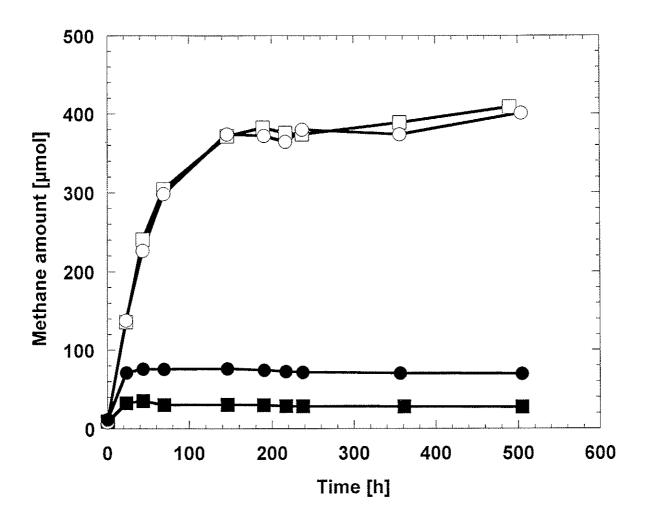
Figure 9. Methane production during reductive dechlorination of PCE and TCE under saturating and subsaturating conditions. Filled circles: Saturating PCE conditions. Open circles: Subsaturating PCE conditions. Filled squares: Saturating TCE conditions. Open squares: Subsaturating TCE conditions.
