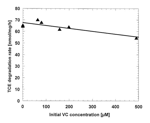
Figure 6. TCE degradation as a function of the initial VC concentration. The initial TCE concentration was  $7.3~\mu M$ .
