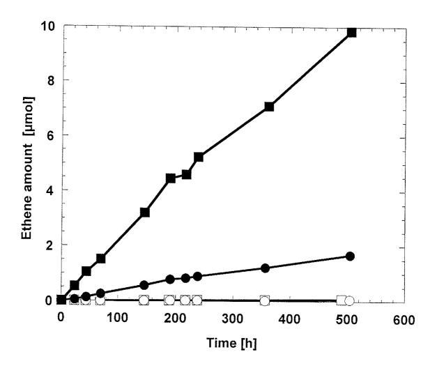
Figure 8. Ethene production during reductive dechlorination of PCE and TCE under saturating and subsaturating conditions. Filled circles: Saturating PCE conditions. Open circles: Subsaturating PCE conditions. Filled squares: Saturating TCE conditions. Open squares: Subsaturating TCE conditions.
