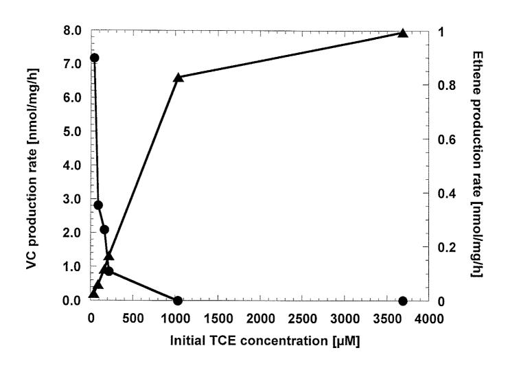
Figure 10. VC and ethene production rates as a function of initial TCE concentration. Filled circles: VC. Filled triangles: ethene.
