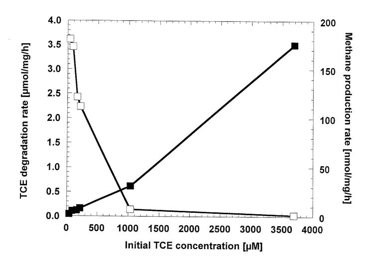
Figure 11. Methane production rates and TCE degradation rates as a function of initial TCE concentration. Filled squares: TCE. Open squares: methane.
