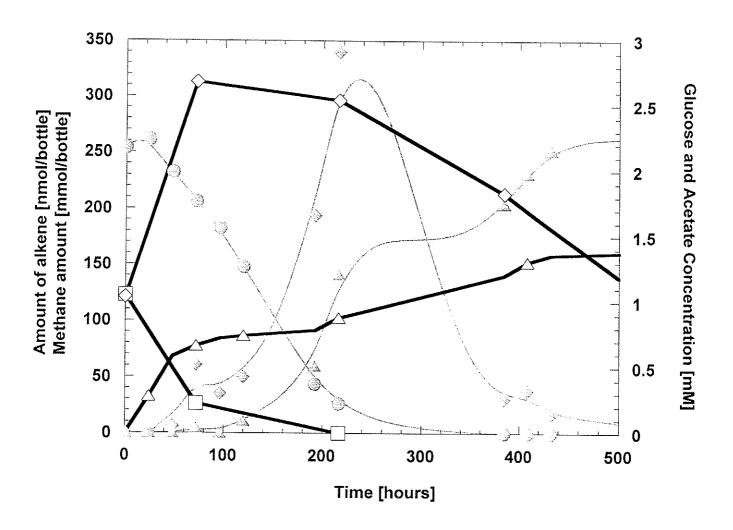
Figure 2. Methane production and glucose and acetate utilization during the complete degradation of TCE to ethene by an enriched groundwater culture using glucose as the carbon source. Filled circles: TCE. Filled diamonds: VC. Filled triangles: ethene. Open squares: glucose. Open diamonds: acetate. Open triangles: methane.
