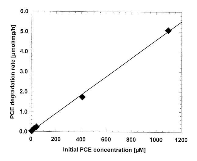
Figure 3. PCE degradation rate as a function of initial PCE concentration.
