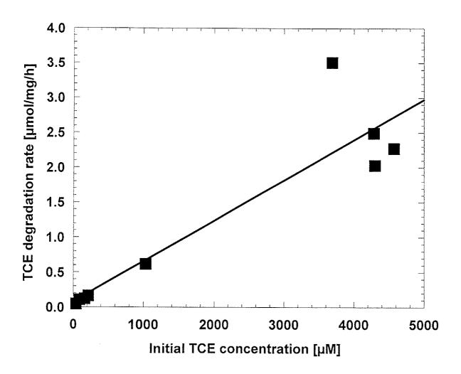
Figure 4. TCE degradation rate as a function of initial TCE concentration.
