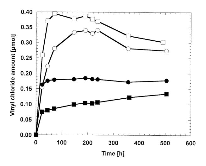
Figure 7. VC production during reductive dechlorination of PCE and TCE under saturating and subsaturating conditions. Filled circles: Saturating PCE conditions. Open circles: Subsaturating PCE conditions. Filled squares: Saturating TCE conditions. Open squares: Subsaturating TCE conditions.
