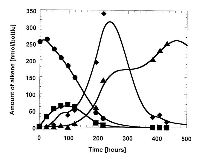
Figure 1. Complete degradation of TCE to ethene by an enriched groundwater culture using glucose as the carbon source. Filled circles: TCE. Filled squares: cis-DCE. Filled diamonds: VC. Filled triangles: ethene
