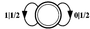
FIG. 6. The \epsilon -machine for the hidden Markov model of Fig. 2. The internal entropy rate h_\mu^X and the statistical complexity C_\mu again vanish since there is a single causal state.
