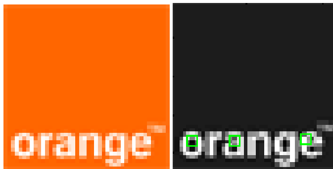
Figure 6.1: This shows a logo that produces an insufficient number of keypoints to be reliably used for image matching. The left image is the original logo; the right image shows the logo after the feature generation step, with keypoints indicated.
