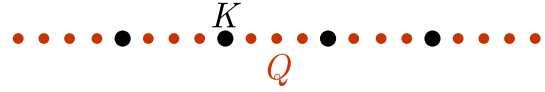
FIG. 8. Reciprocal lattice in 1d for a four-site cluster. K labels the reciprocal lattice vector for the original lattice and Q labels the reciprocal lattice vector for the superlattice. More precisely, K_s = \frac{2\pi}{a}s and Q_s = \frac{2\pi}{La}s , where a is the lattice constant of the original lattice, L = 4 here and s \in \mathbb{Z} .
