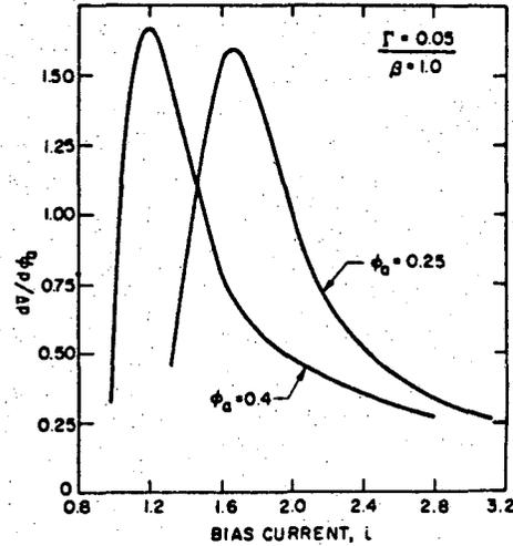
Fig. 4.  $d\bar{v}/d\phi_a$  vs.  $i$  for  $\phi_a = 0.25$  and  $0.4$ .
