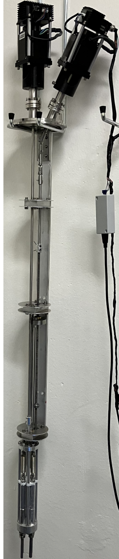
Figure 3.1. Picture of entire sample changer stick.
