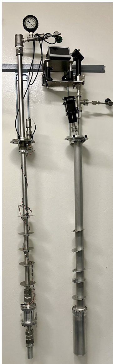
Figure 4.1. A photograph of the two photochemistry sample sticks mounted vertically. On the left is the passive design sample stick and on the right is the tumbler design sample stick.
