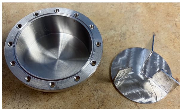
Figure C.3. Aluminum sample can with tumbler blade inserts.
