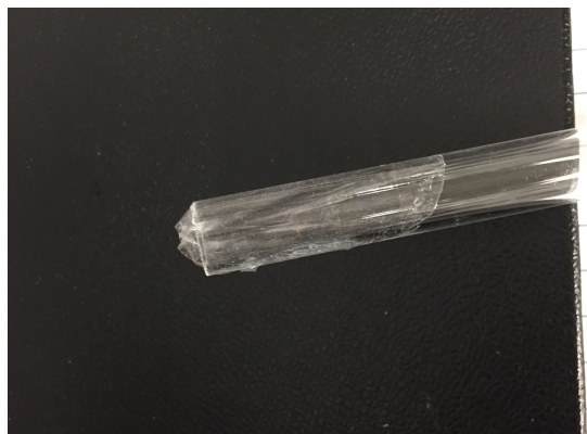
Figure 6.5. Polystyrene film wrapped around quartz tube.
