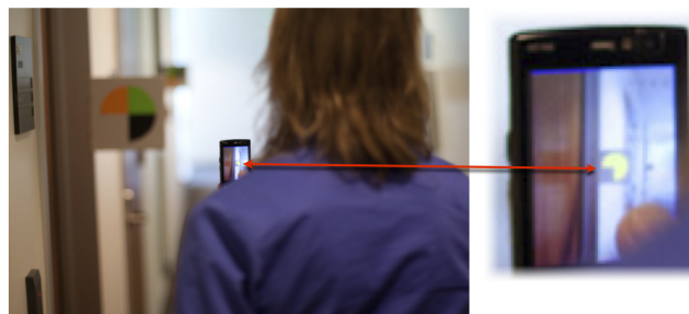
Fig. 1. Our color marker system, tested in the Env3 environment. The right image shows the view from the viewfinder; the pie-shaped color marker is displayed in yellow, signaling that detection has occurred.
