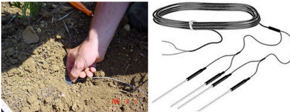
Figure 4. Instrumentation needed to measure soil heat flux (G). On the left, a soil heat flux plate is being inserted at a depth 0.05 m. The soil thermocouples, on the right, are inserted at an angle from about 0.04-0.01 m depth where the cable end is at the deeper depth. The thermocouples measure the temperature change from the beginning to the end of the sampling period (30 min).
