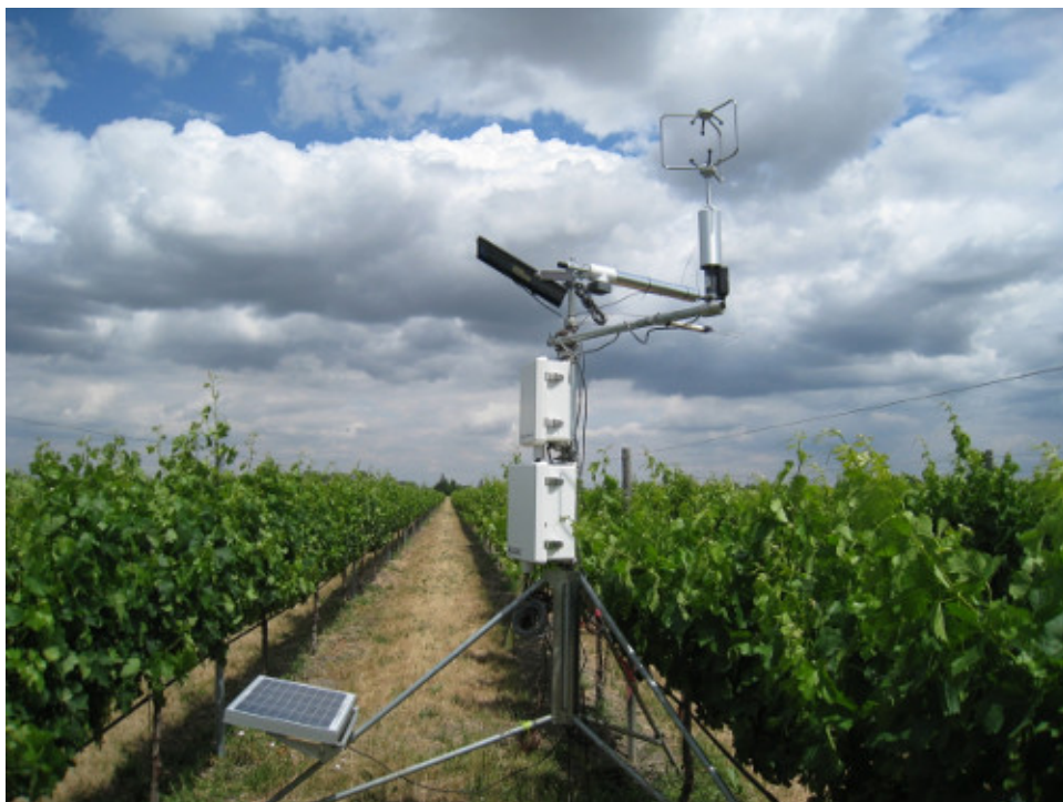
Figure 1. Solar powered field station established in a vineyard in California to measure surface renewal with a sonic anemometer for calibration using eddy covariance.
