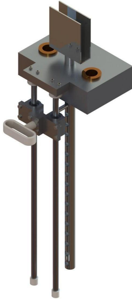
Figure 2: Top: The modified weight selector pin carrier, with large handle. Bottom: The full pin assist system.
