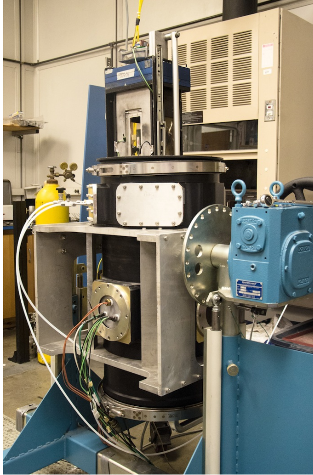
Figure 3.4: Pressure chamber and tunnel in vertical position.
