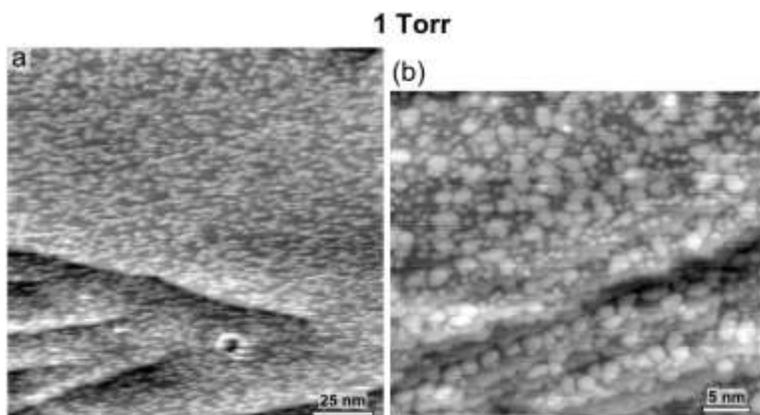
**Figure S3** STM image at 1 Torr of CO. The number of 3-atom clusters decreases substantially while larger clusters form on the surface Imaging parameters: [ $V_b = 0.9$  V;  $I_t = 0.2$  nA] in (a), [ $V_b = -1.15$  V;  $I_t = 0.2$  nA] in (b).
