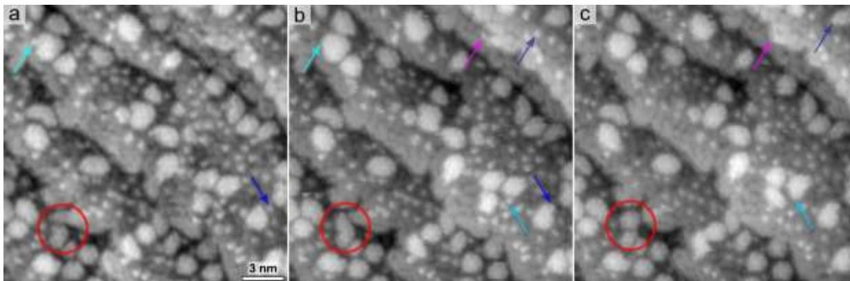
**Figure S2** Evolution of Cu(111) surface under 0.2 Torr of CO at RT. Cluster formation stages are highlighted with red circles. Arrows show cluster ripening. Time between displayed frames:  $\sim 180$  s [ $V_b = -1.5$  V;  $I_t = 0.2$  nA].
