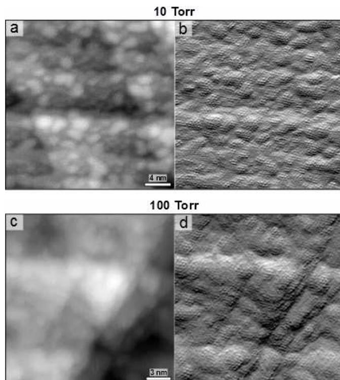
**Figure S4** CO induced cluster formation on Cu(111). STM images of CO covered Cu clusters under (a) 10 Torr of CO [ $V_b=0.15$  V;  $I_t=0.8$  nA] and (c) 100 Torr of CO [ $V_b=0.15$  V;  $I_t=1.1$  nA]. (b) and (d) are derivative images of (a) and (c), respectively.
