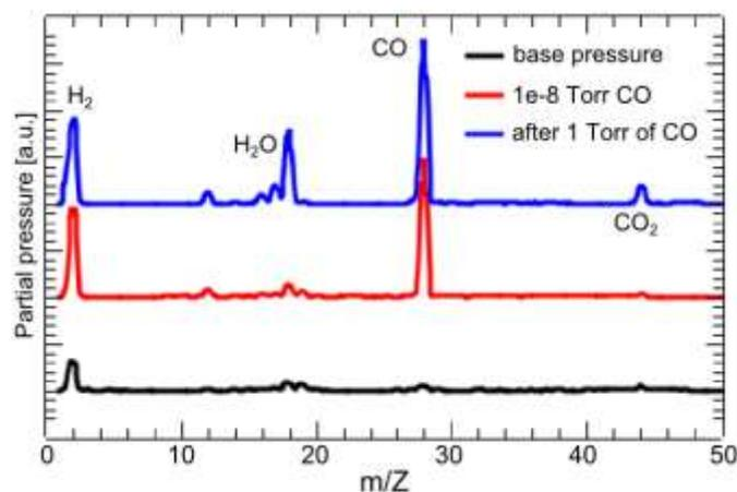
**Figure S8** Mass spectrum acquired in the STM chamber at the base pressure of  $1 \times 10^{-10}$  Torr, and reference spectrum under  $1 \times 10^{-8}$  Torr of CO (black and red curves). After the chamber is pumped down to  $1 \times 10^{-8}$  Torr in a few minutes following CO experiments at 1 Torr, residual gases H<sub>2</sub>, H<sub>2</sub>O, CO, and CO<sub>2</sub>, are observed. After a few minutes more, a pressure of  $2 \times 10^{-9}$  was
