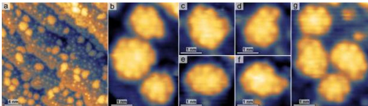
**Figure S1** (b-g) Different clusters observed in (a). In all of the clusters, the edges are decorated by maxima due to CO molecules. Only the corner molecules have high contrast in the STM images [ $V_b = -1.5$  V;  $I_t = 0.2$  nA].
