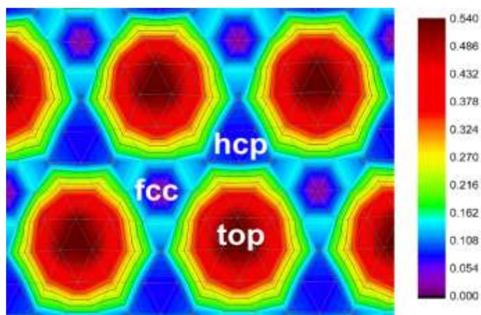
**Figure S5** Top view of the potential energy surface for the Cu adatom on Cu(111) surface. The smallest diffusion barrier is 0.14 eV for Cu hopping from fcc to hcp sites. The bar shows the color-coded relative energies in eV.
