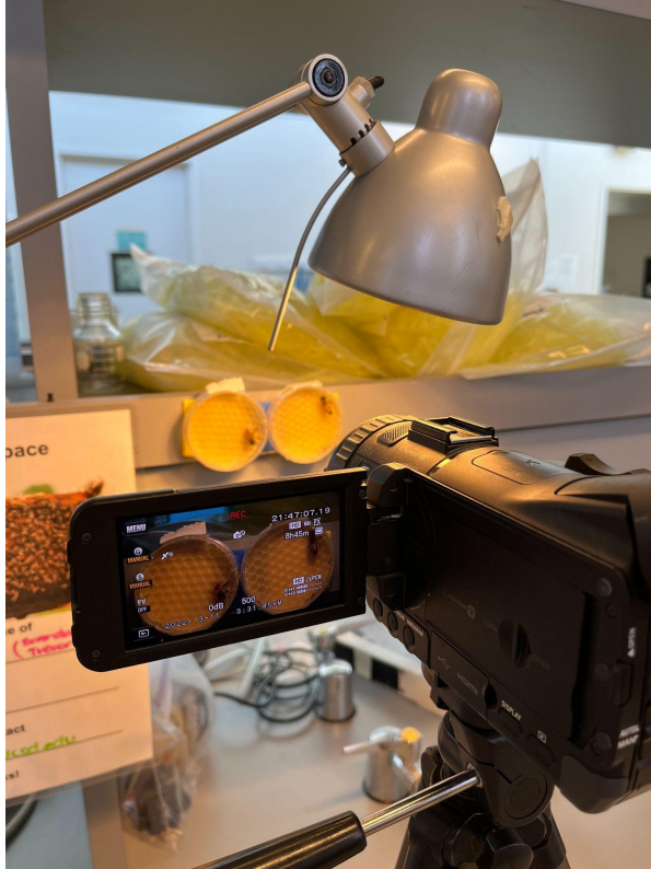
Figure 3. Self-grooming behavioral assay setup. Two Petri dishes with press-in beeswax comb foundation are mounted vertically so they were level with the camcorder. An LED lamp was placed above to illuminate the video further.
