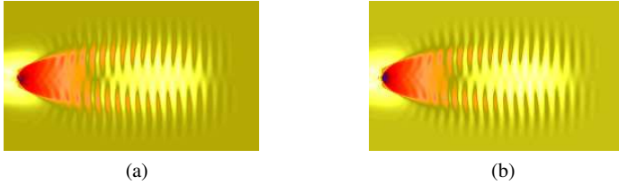
FIGURE 4. Contour plots of the wake fields produced by OSIRIS (a) and VORPAL (b) for a_0 = 4 with second-order particle shapes ( i.e. , second-order field interpolation and second-order current deposition).
