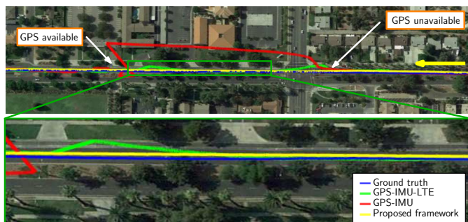
Fig. 7. Vehicle's estimated trajectory from the GPS-IMU system versus our proposed framework when GPS signals become unavailable and then available are specified. As can be seen, the GPS-IMU solution drifts in the absence of GPS signals. In contrast, our proposed framework does not exhibit such drift as cellular signals are used as an aiding source to the IMU. Image: Google Earth.
