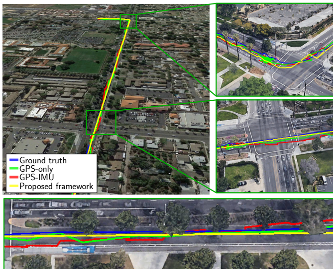
Fig. 6. Experimental results in an urban environment. The vehicle's estimated trajectory with our proposed framework is compared against the estimated trajectory with a GPS-only and a GPS-IMU system. The ground-truth was obtained with an expensive GPS-IMU system with RTK. Experimental results indicate a 2.80 m RMSE for the proposed approach. Image: Google Earth.
