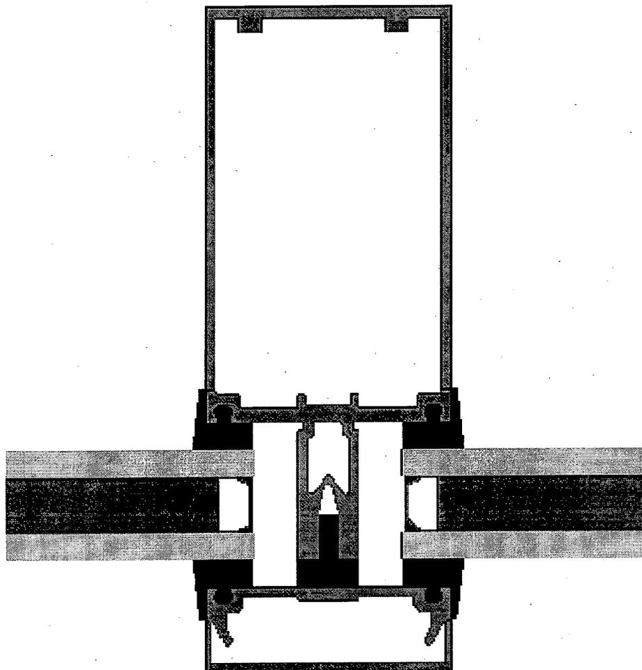
Figure 3. Frame cross section without fastener, shown with Pseudo IG.
