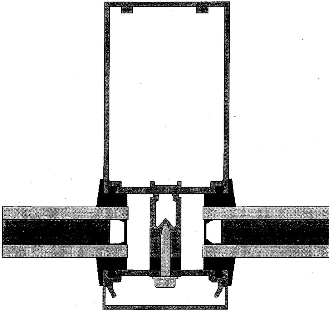
Figure 2. Frame cross section with fastener, shown with Pseudo IG.
