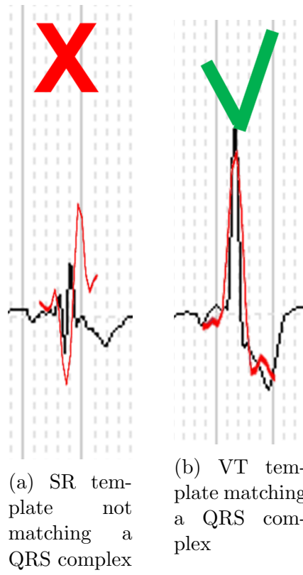
Figure 7.6: Comparison between a template and a QRS complex before and after update
