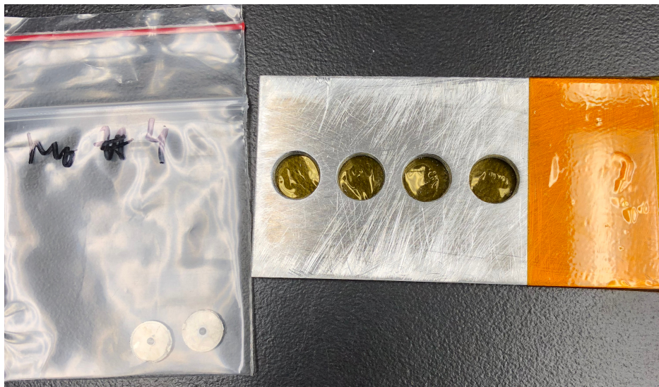
Figure 3.15: Custom target holder for the measurement of the ^{98}\text{Mo}(\text{n},\gamma)^{99}\text{Mo} cross section at four energy locations near 2.7 MeV.
