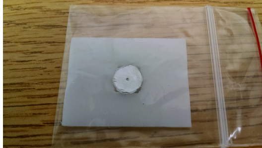
Figure 3.11: Sample holder used for the Berkeley HFNG. The zinc (visible) foil is co-loaded on top of reference indium foil, ready for irradiation.
