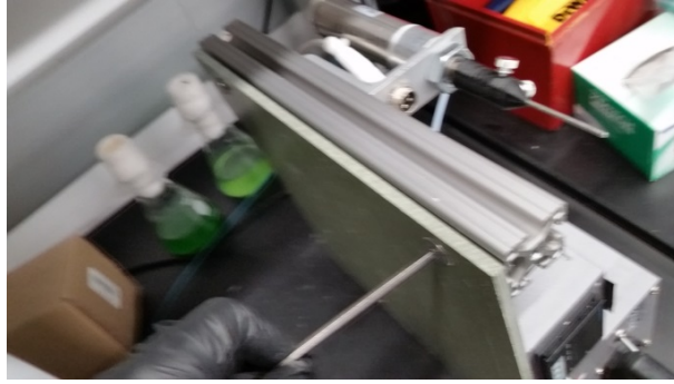
Figure 4.16: Tighten screws to secure rail in place
