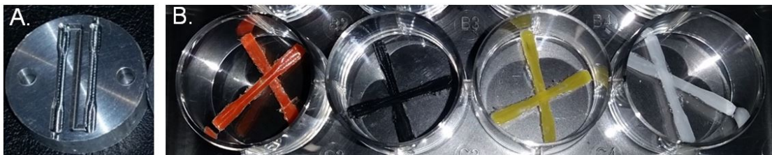
Figure 4.10: A) aluminum dog bone injection mold used during the current study, B) successfully injection molded PCL samples 5-8 (from left to right); Doxorubicin, MWCNT, Ferrocene, and pure PCL.
