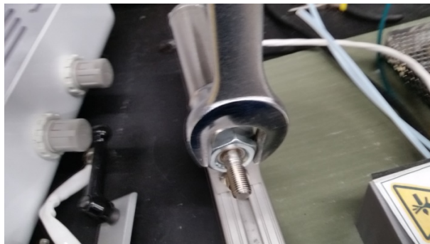
Figure 4.20: Cylinder secured using included nut
