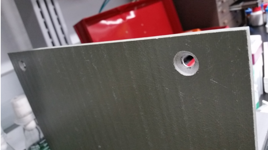
Figure 4.14: Deep countersunk holes in base plate using step drill or countersink drill
