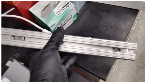
Figure 4.15: Insert rail fasteners into rail
