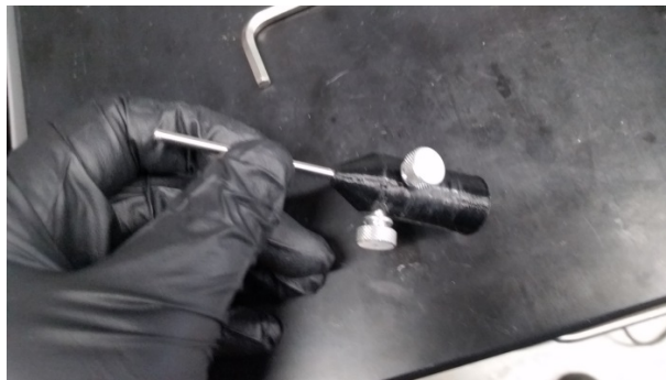
Figure 4.22: Gauge pin inserted into shaft collar with threaded 8-32 thumb screws securing it in place
