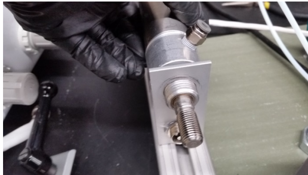
Figure 4.19: Cylinder mounted in place
