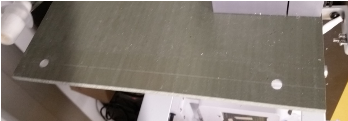
Figure 4.13: Mark FRP base plate as shown above
