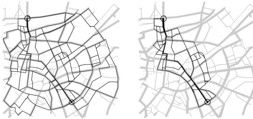
Figure 2. 2 System optimum without and with restrictions on the length of a path
