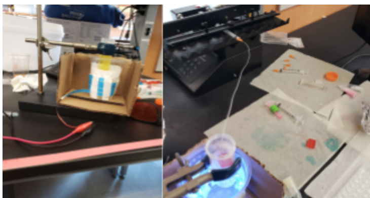
Figure 9 - Setup using pump and UV Light to create microparticles
