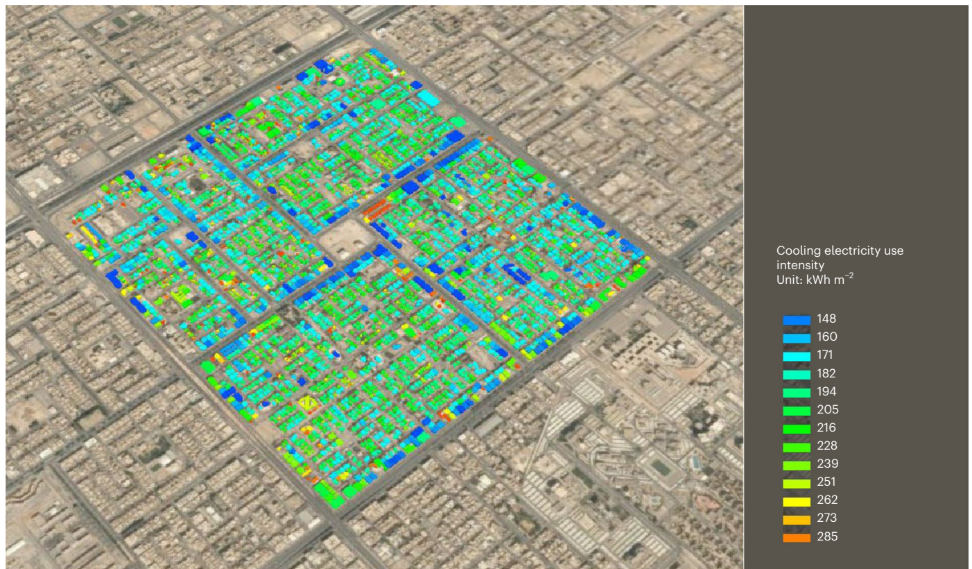
Fig. 2 | Cooling load of the buildings. Distribution of the calculated annual cooling load of the buildings under reference conditions.
