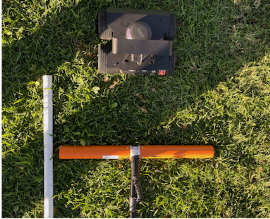
Figure 3.4: In field tests to identify EMI interference, the sensor (orange cylinder) was operated in a manual configuration to record a series of measurements at multiple distances and fixed orientation (either 0^\circ or 90^\circ ) from the robot, over diverse fields. Here we show an instance from testing over irrigated turf at d_h = 25 mm and \theta = 0^\circ .
