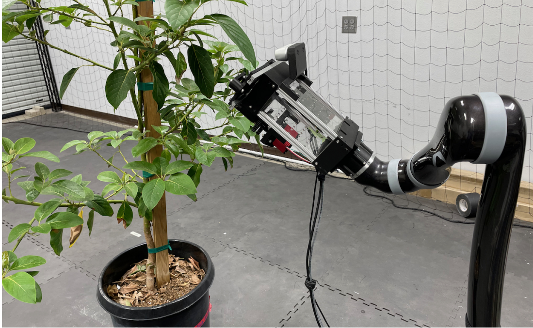
Figure 5.1: The a custom-built end-effector developed in Chapter 4 mounted on an off-the-shelf 6-DOF robotic arm to detect, localize and cut leaves at their stem.
