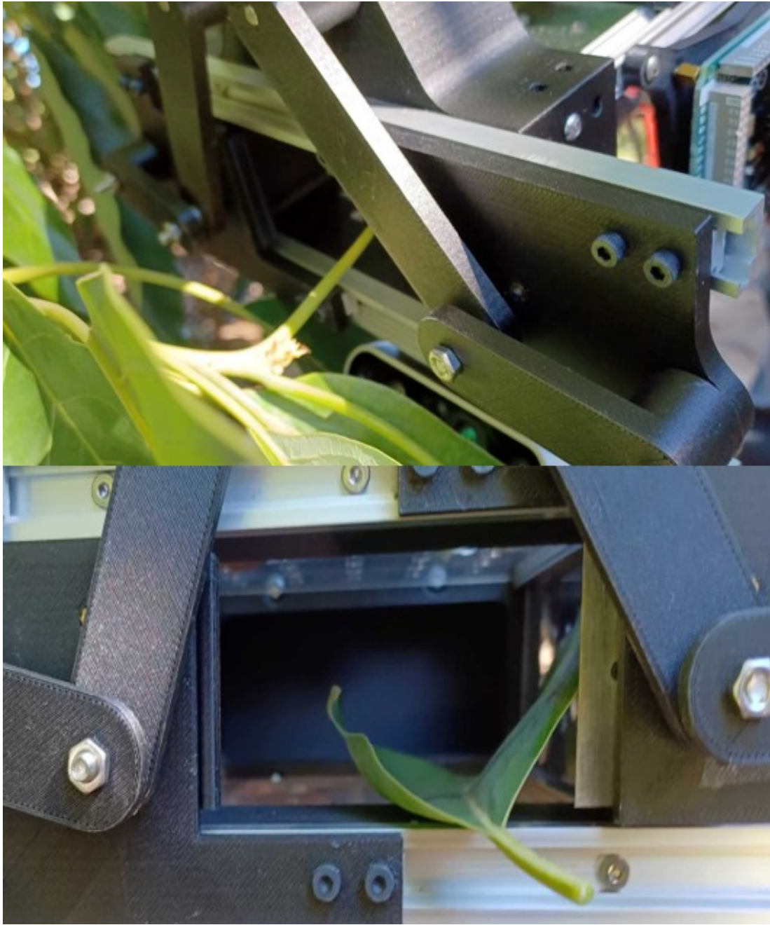
Figure 4.6: For the field leaf cutting tests, the battery-operated end effector was manually placed about the stem and activated by a button press on the on-board microcontroller (top). Normally, the cut leaf falls into the end effector for retention, but the stem was pulled out for visual inspection (bottom).
