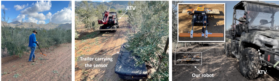
Figure 3.2: Current and envisioned soil moisture (SM) survey techniques using electromagnetic induction (EMI) sensors in traditional and precision agriculture. Current methods include manually-collected data obtained by walking the sensor in the field (left panel), and data obtained by a person driving a field vehicle that pulls the sensor secured on a trailer (central panel). Both methods are labor-intensive. In contrast, the proposed robotic method seeks to automate this process via the use of small and portable agricultural robotics (right panel). The robot prototype is significantly smaller than the ATV and sensor trailer. Due to its small size, it is able to navigate closer to the drip-lines at the base of the trees and exert more control over the spatial component of apparent Soil Electrical Conductivity (ECa) measurements. The robot contains all necessary equipment to perform the measurement including the EMI sensor, a GNSS receiver, and router to provide a local field network.
