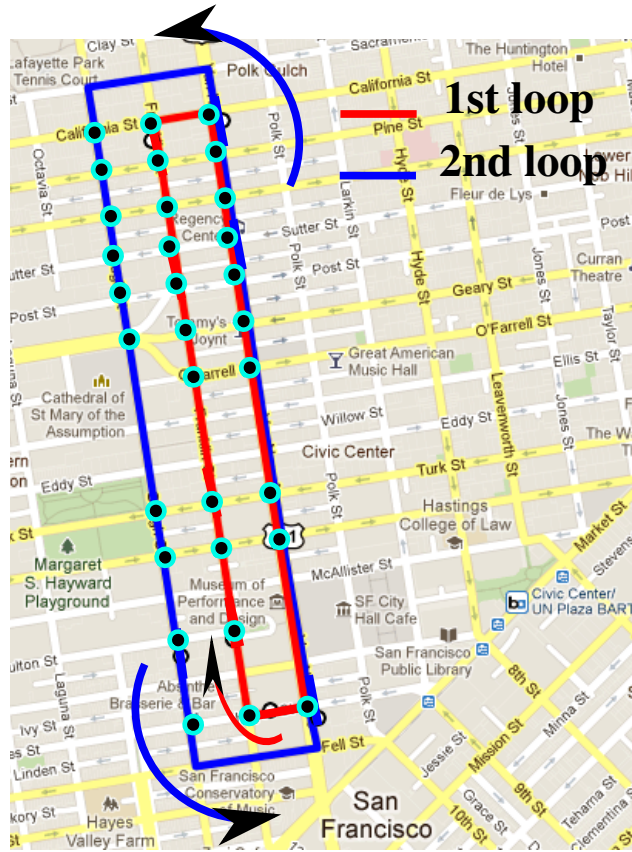
Figure 5.6: Routes of the network used for field test validation. The drivers drove around two distinct loops consisting in Van Ness Ave. South bound and Franklin St. north Bound for the first routes and Van Ness Ave. North bound and Gough St. South bound for the second route. Signalized intersections are indicated with a circle.
