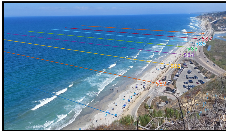
Figure 3: A photo taken from the CoastSnap station at Torrey Pines, showing the MOP lines 581-587 analyzed in this project
