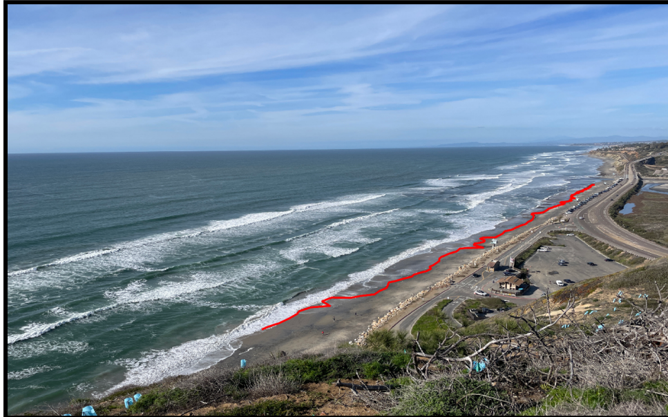
Figure 11: A shoreline from January 2023 mapped using the CoastSnap MATLAB Toolbox. A portion of the mapped shoreline (red line) closest to the camera is deviated in the seaward direction due to a misattribution of the edge of white water as the shoreline.
