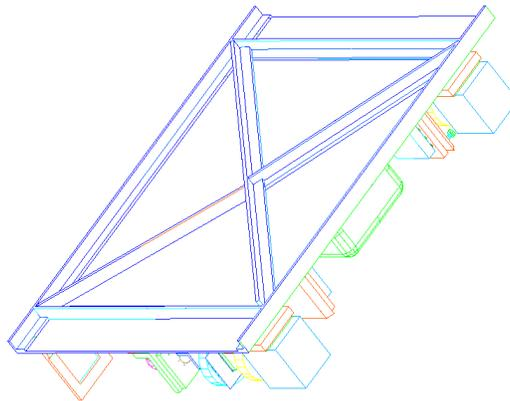
Figure 7-3 The System Support Frame and Plate
