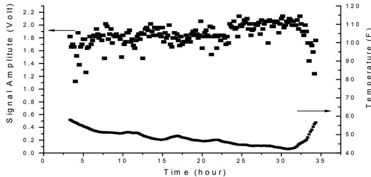
Figure 8-1 Signal Amplitude tested in Clear Weather
