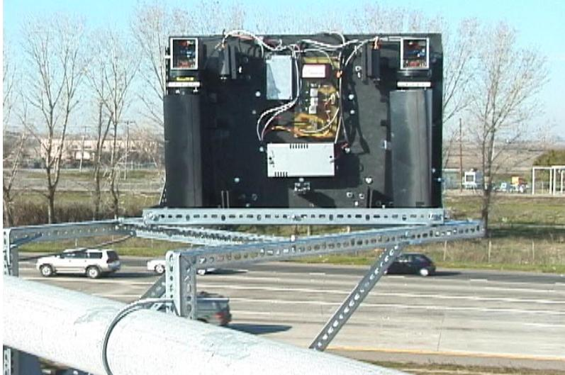
Figure 8-4: Detection System Mounted Above the Highway.
