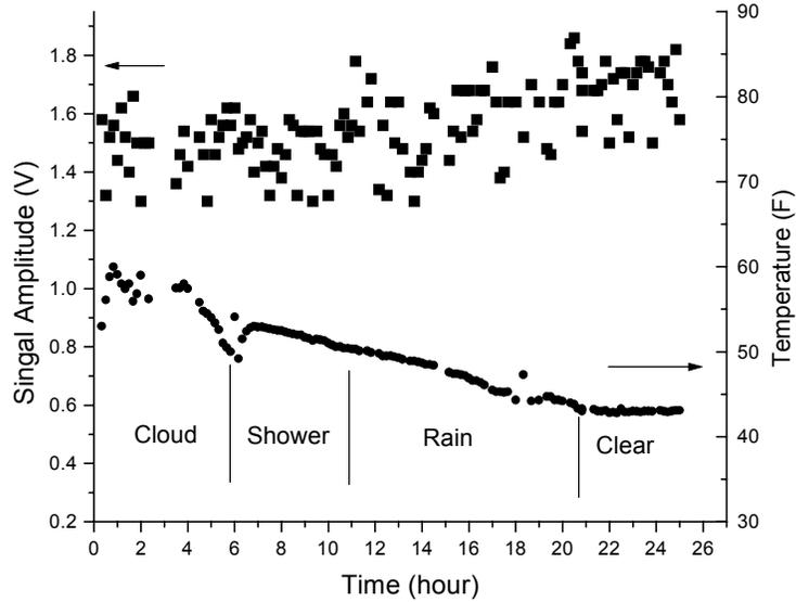
Figure 8-2 Signal amplitude for different weather conditions.
