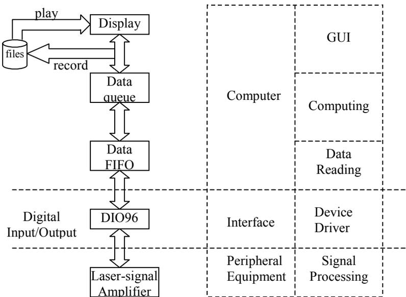
Figure 2-3 system architecture
