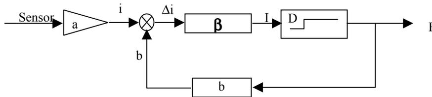
Figure 5-1 feed back diagram
