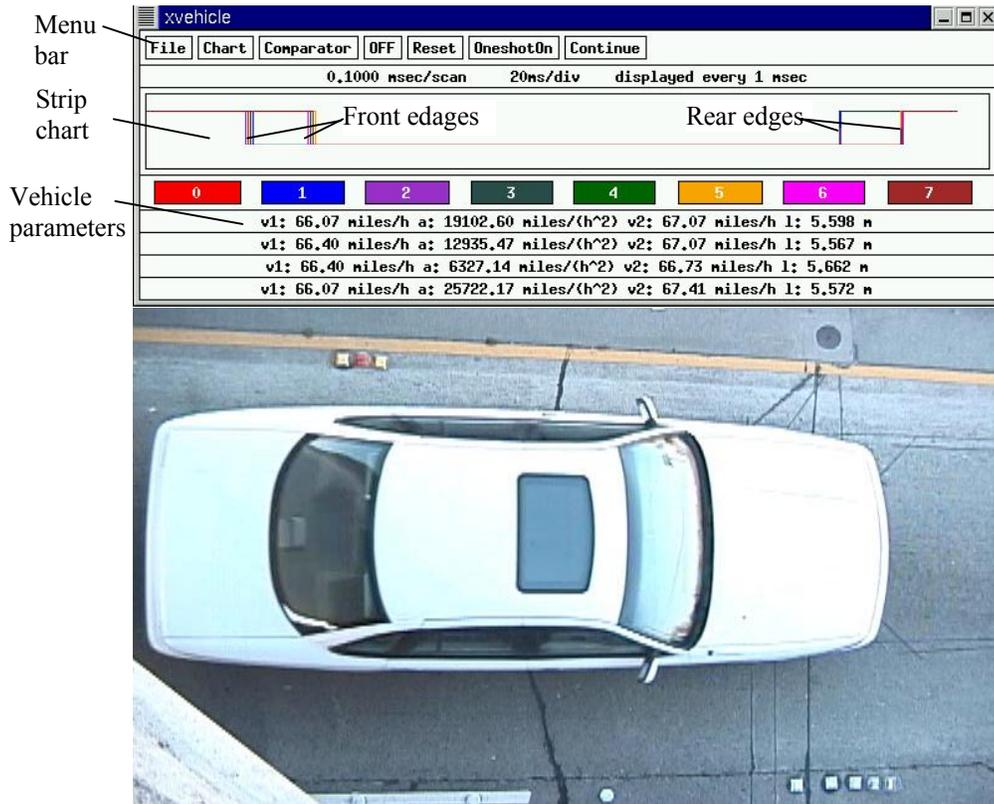
Figure 8-5: Test Results for a Passenger Car.
