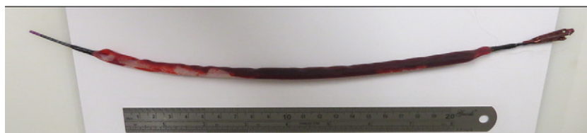
Figure 1: In vitro flow model experiments. (a) Graph shows doxorubicin (DOX) filtration over the course of 60 minutes from porcine whole blood (0.05 mg/mL DOX) ( n = 6 ). Data are presented as mean \pm standard deviation. (b, c) Photographs of the Chemofilter device before (b) and after (c) the flow model experiment.
