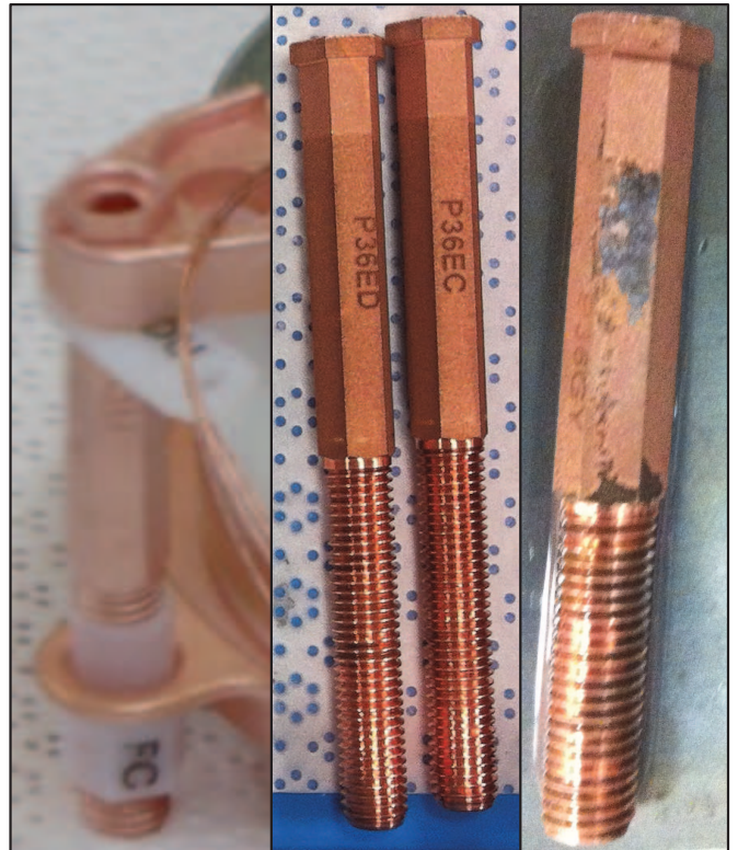
Figure 2: Hollow hex rods: Part P33QU made from OFHC copper in detector unit P34Y7 (left panel), photographed through glovebox window. Parts P36ED and P36EC made from electroformed copper (center panel). Part P36GY made from electroformed copper that has had a mishap during fabrication (right panel).
