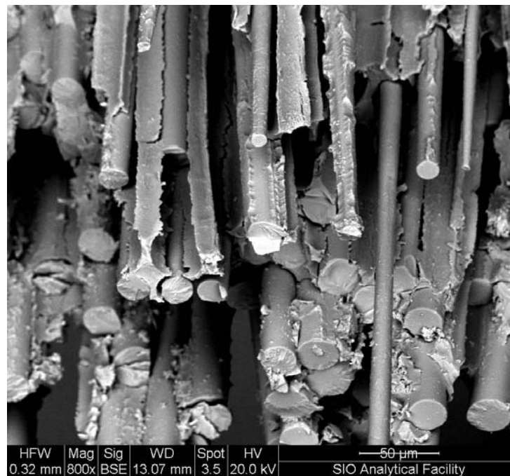
Figure 162. SEM of failed dry tensile specimen exposed to 80°C immersion. Tested after post-conditioning.
