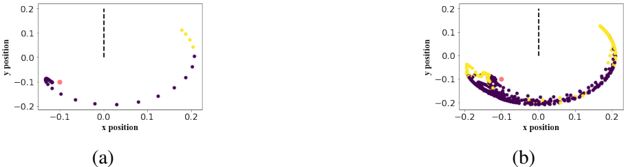
Figure 4.3: Sample trajectories for the Reacher environment (Figure 4.2a). The yellow points are the choice of safe policy and the brown points are the choice of free policy. The top dotted line is the constraint, the red point is the random target. (a) One trajectory of the agent. (b) A large subset of trajectories of the agent.
