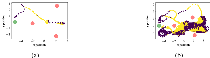
Figure 4.4: Sample trajectories for the Racecar environment (Figure 4.2b). The three red points are the random obstacles. The blue point is the destination. The yellow point means the agent chooses the safe policy at the current state, whereas the brown point means the free policy. (a) One trajectory of the agent. (b) A large subset of trajectories of the agent.
