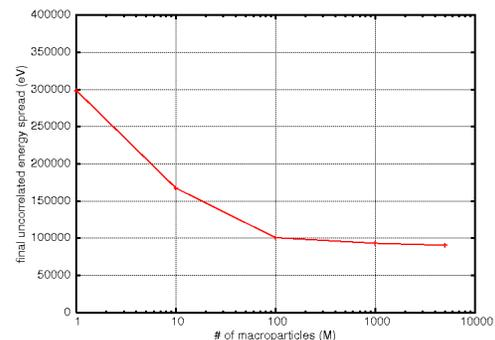
Figure 4: Final electron beam energy spread as a function of number of macroparticles.
