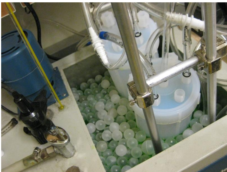
Fig. 4. Two experiments set up in temperature controlled reactor bath with Teflon balls and ethylene glycol for insulation
