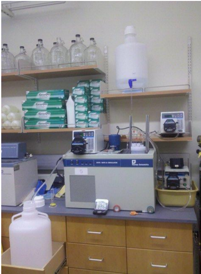
Fig. 20. Flow-through setup with influent above bath and effluent below/adjacent. Peristaltic pumps pump seawater in and out at equal rates so that solution volume remains constant. Seawater flows 13 mL/min, and a third pump mixes solution inside the vessel.
