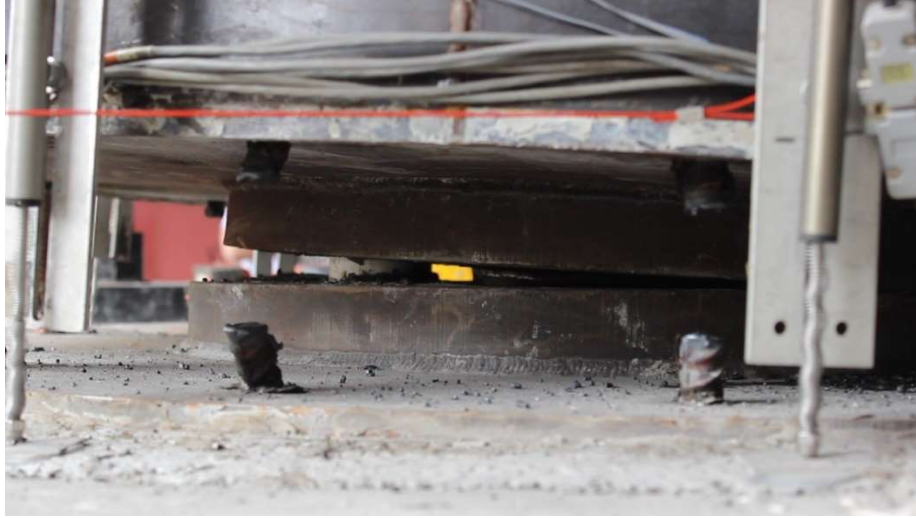
Figure 9.27: Opening of rocker hinge at the beginning of free-vibration test 4
