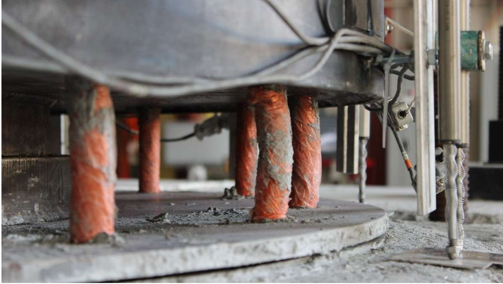
Figure 9.3: Extreme north rebar bent in ungrouted gap of Specimen 1
