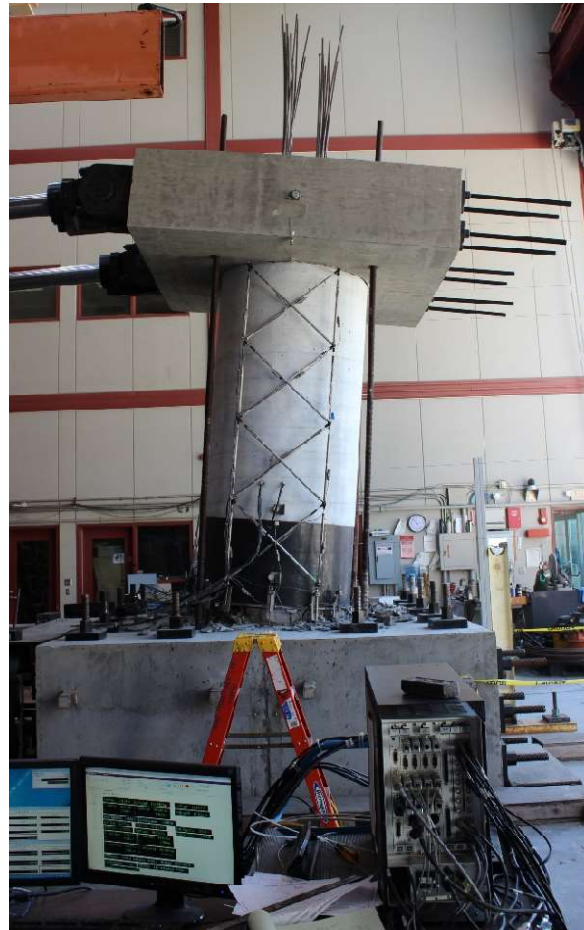
Figure 9.11: Picture of Specimen 1 at 10% drift ratio
