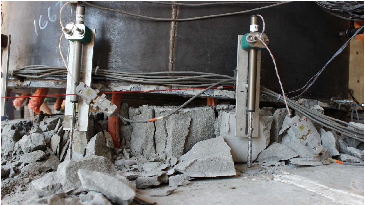
Figure 9.9: Picture of west side of sacrificial region of Specimen 1 at -10% drift ratio
