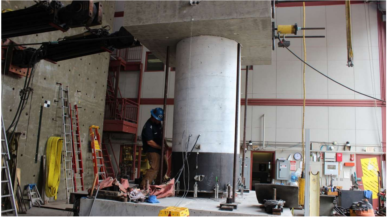
Figure 8.8: Picture of free-vibration tests of Specimen 1
