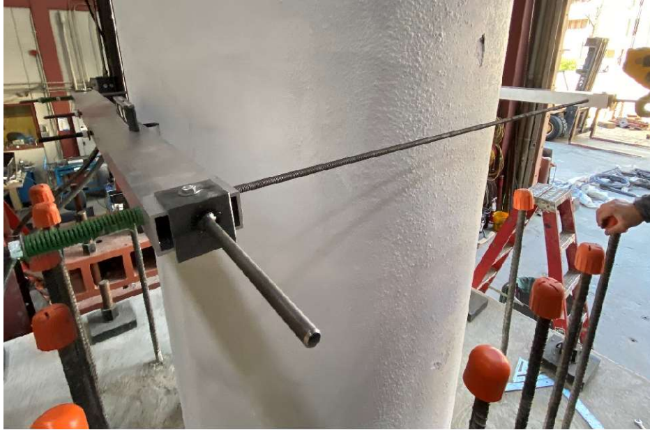
Figure 3.14: Picture of aluminum mounting brackets for the linear displacement potentiometers to measure flexural and shear deformations
