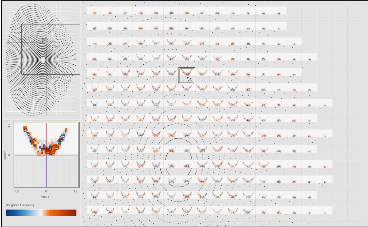
Figure 2.1. A visualization of distribution functions for the time-varying GTS data. The visualization is a screenshot of the visualization system presented in Chapter 4. These distribution functions represent signed perturbations of the phase-space particle distribution function, as explained in Chapter 4 and further in Appendix A.1.2. The purpose of this figure is to highlight some of the characteristics which motivate the use of non-parametric models.
