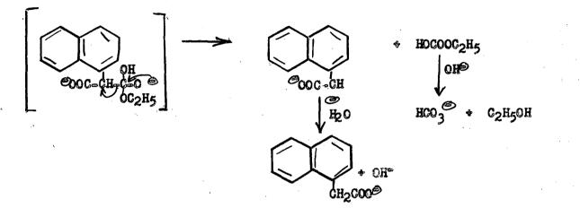
The carbon-carbon bond in the above complex is undoubtedly weakened by the repulsion between the two negatively charged ends of the molecule, thus facilitating the carbonate cleavage. This weakening effect is not present in the hydrolysis of the diester, and is perhaps the reason why we do not get this cleavage during this first hydrolysis step.
