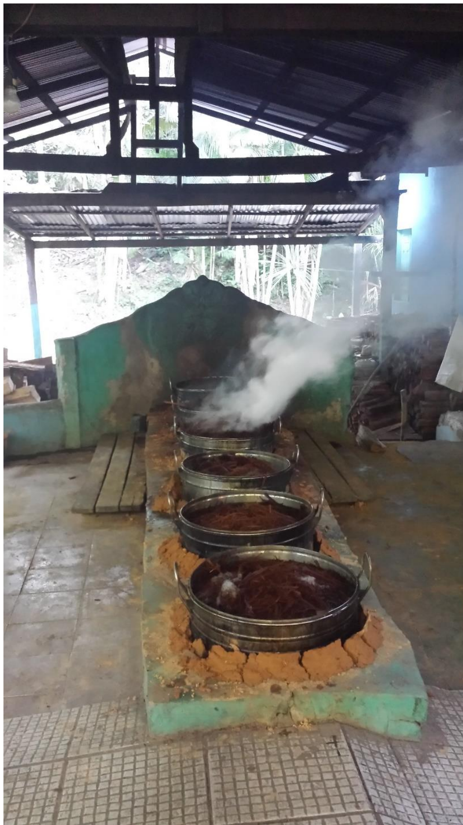
Image 20: Two large wood burning ovens heat twelve 60-gallon cooking pots at the “feitio”. 88
