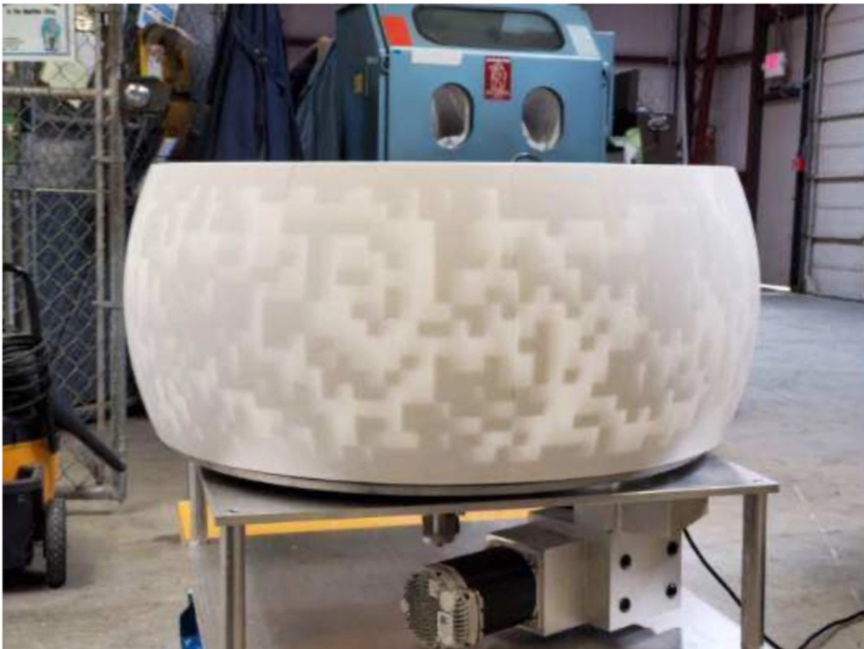
Figure 5.3. A photo of the 3D-printed mask installed on the system. It sits on a circular platform on top of a rectangular frame. The motor is mounted under the top of the frame and connected to the circular platform.
