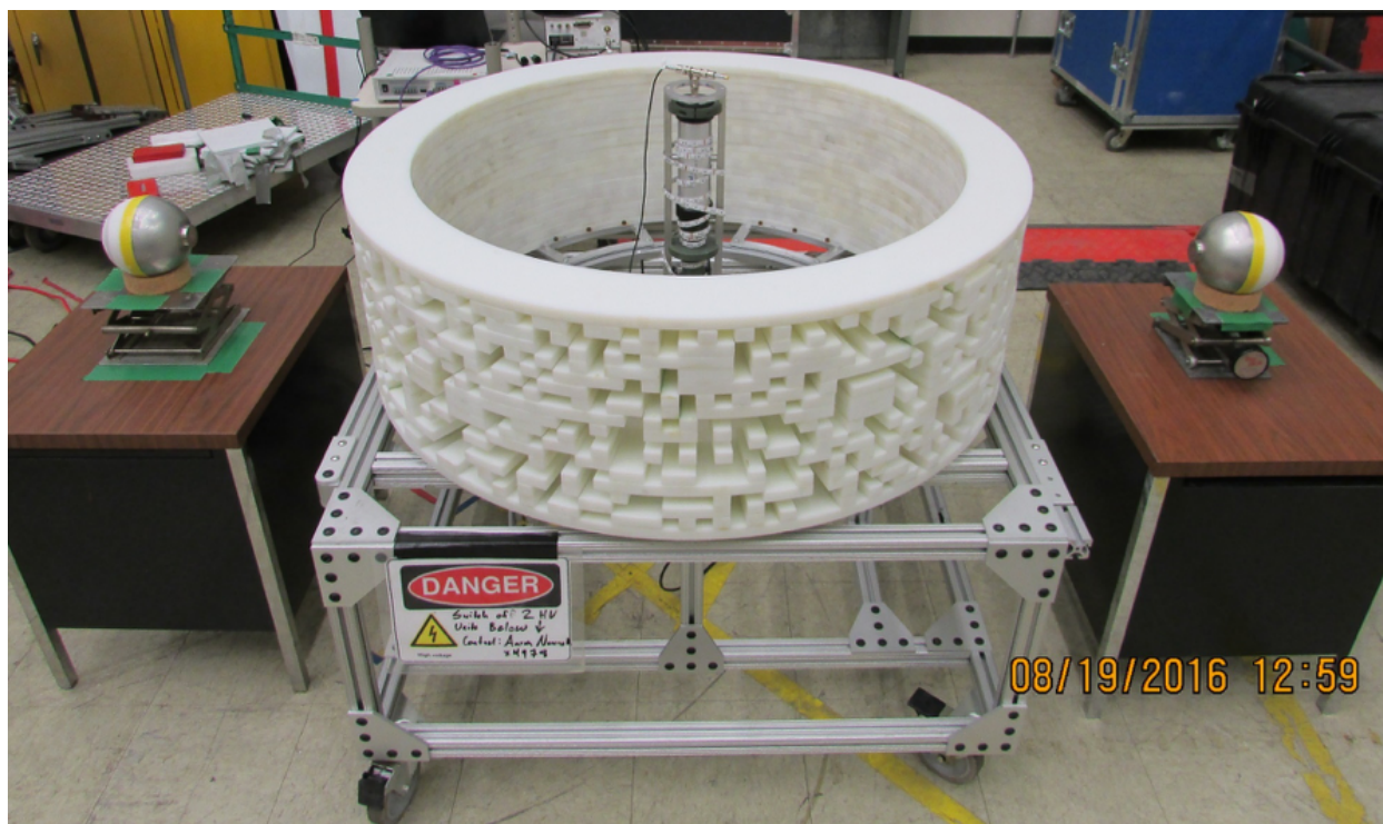
Figure 3.7. CONFIDANTE with the LLNL PuO 2 hemispheres.
