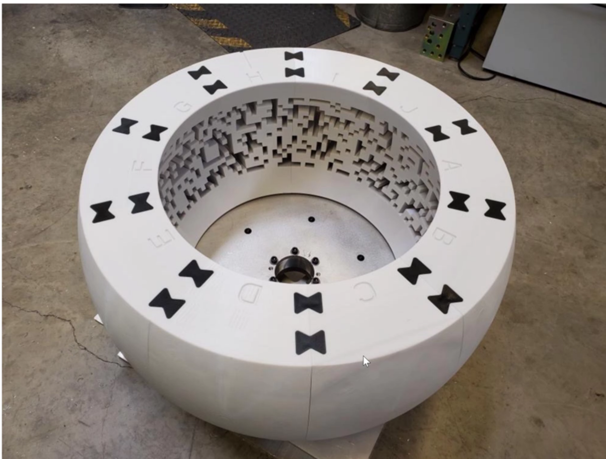
Figure 5.1. A photo of the 3D-printed mask from overhead. Small 3D-printed wedges (in black) fit into the top surfaces of 10 arc segments of the mask to keep them locked together.
