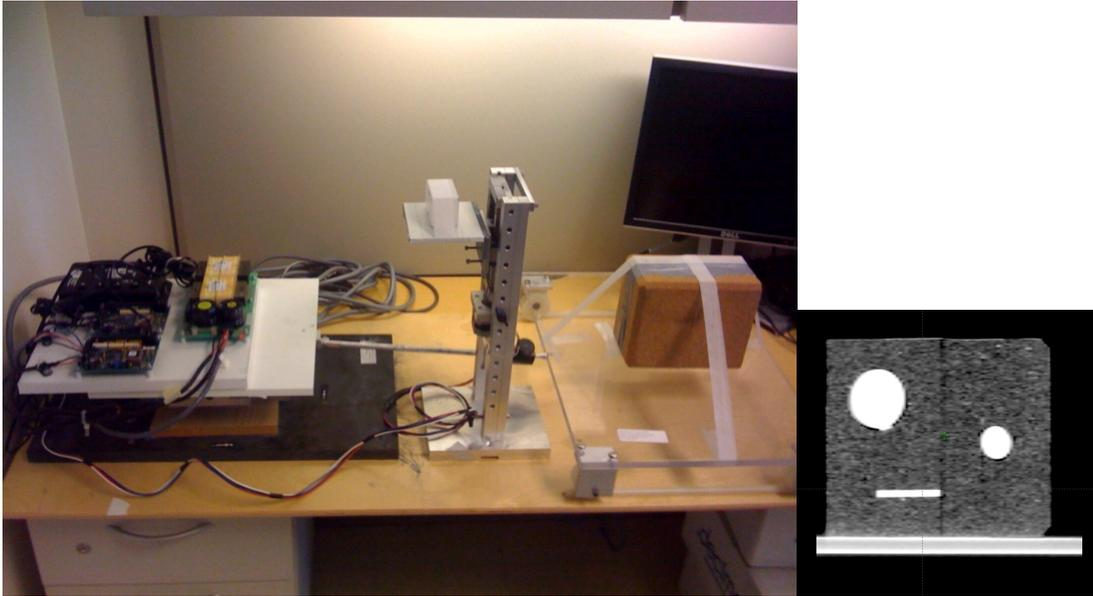
Figure 2.5: A picture of the physical phantom used (left). The sagittal CT slice on the right shows the objects embedded in the cork block.
