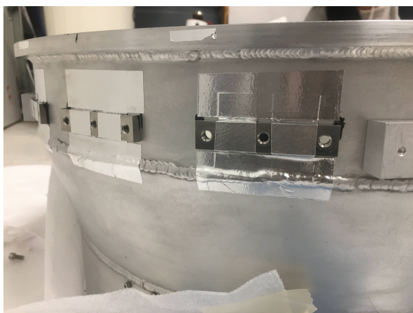
Figure 3.13: This photo shows the nut plates for the heatstraps taped with aluminum tape to the outside of the 4 K taper shell. This was strong enough to solidly hold the nut plates in place. Photo courtesy of Lindsay Ng Lowry.
