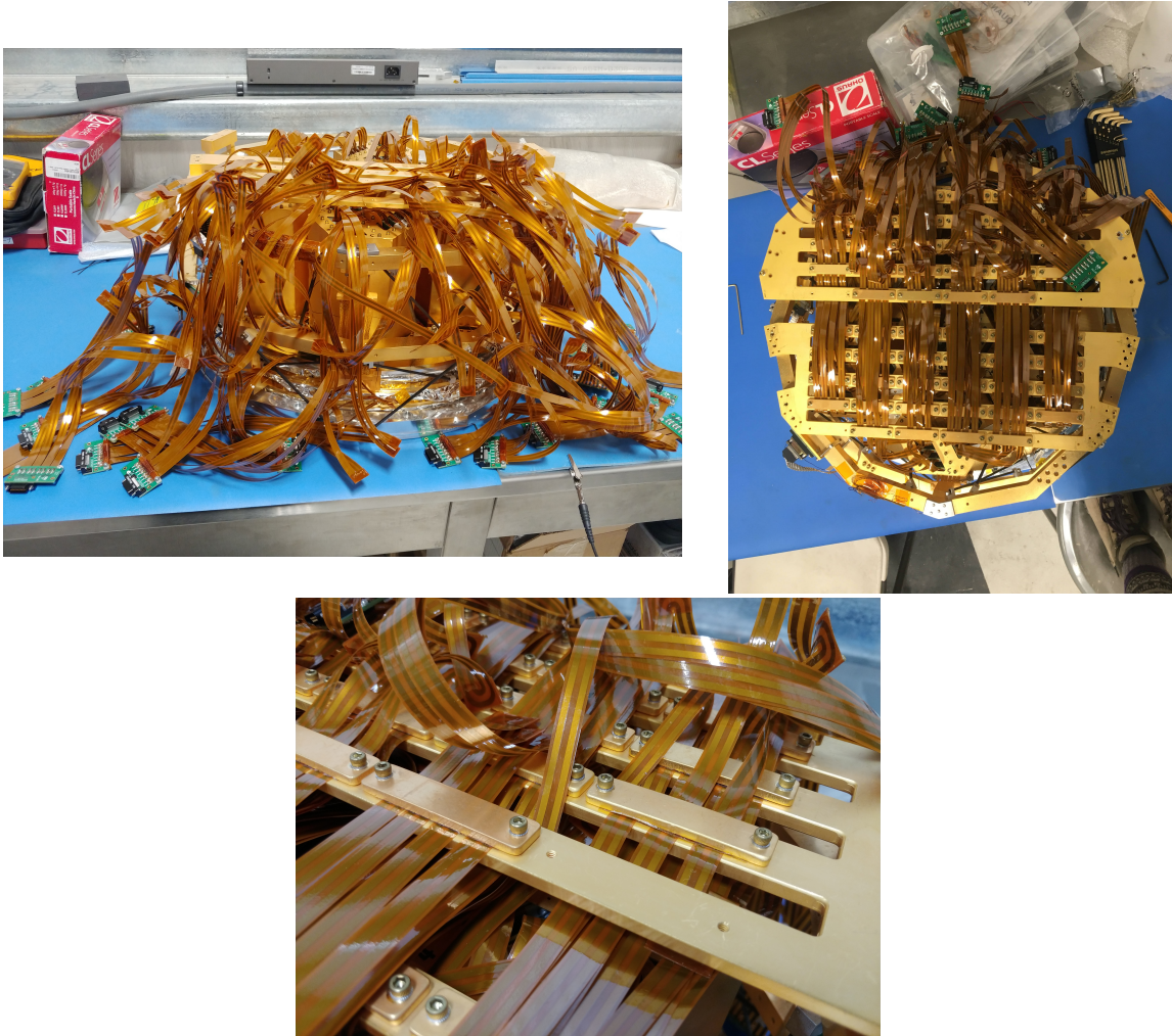
Figure 3.6: Top left: This photo shows the FPT facing down onto the table with all the striplines before they are heatsunk. Top right: This photo shows the striplines after being heatsunk to both the 1 K and the 350 mK heatsinks. Bottom: This photo is a close-up that shows how the striplines are clamped to the heatsink rack.
