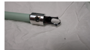
(b) Photo of a broken Al tab
