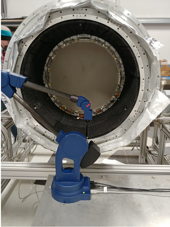
(a) Microscribe mounted on a table
