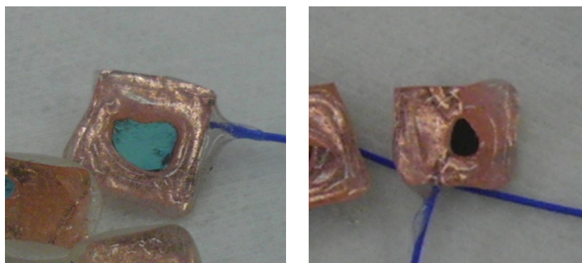
Figure 4.5 Photograph of Cu samples after electrochemical oxidation at constant current densities of 10 ( left ) and 5 ( right ) mA/cm 2 , yielding Cu(OH) 2 and copper oxide, respectively.
