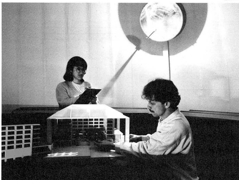
In the facility's interior, Osterhaus and Beltrán conduct performance tests of a shading device for a hotel atrium using the sun simulator, upper right.
