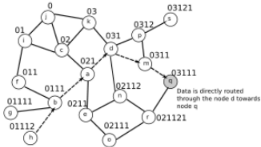
Figure 4.3: Routing Unicast Traffic [1]
